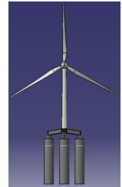
Triple-Spar concept (Lemmer et al., 2016)
