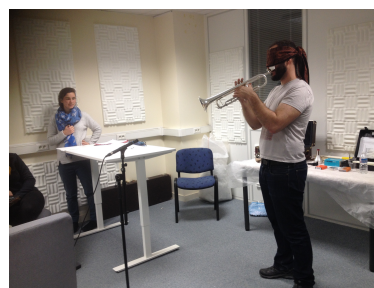
Figure 1. (left): Assembly of the bridges on the mouthpiece of the trumpet. (right): Trumpet player performing an ABX blind test of the bridges in free playing conditions
