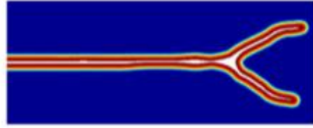
figure 1 : branching of crack path with the TLS method
