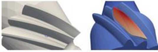
Spiral bevel pinion gear: initial crack location (left) and final crack opening (right)
