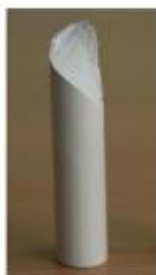
Chalk breakage under torsion
